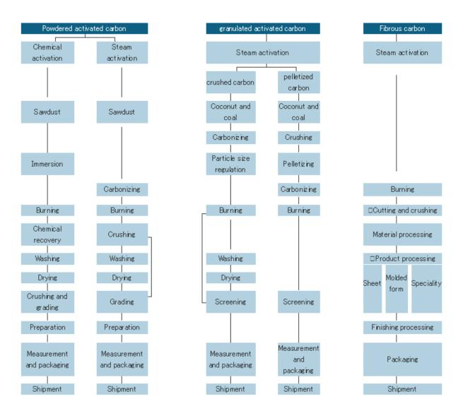
Figure 2.2 Activated carbon production methods [7]
