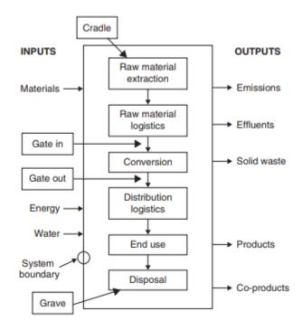
Figure 2.4 Complete life cycle from extraction of raw materials to disposal for product production [21]
