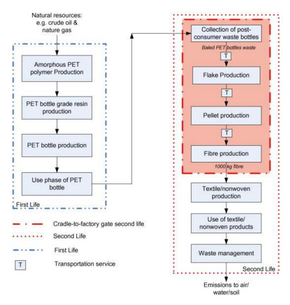
Figure 2.12 Cradle-to-factory gate system boundary of recycling PET fibres from waste bottles, splitting the first life and the second life based on the "cut-off" approach [25]
