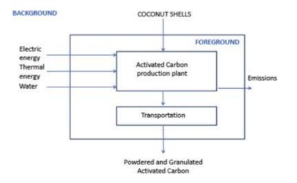
Figure 2.6 System boundaries for the activated carbon production from coconut shells in Indonesia [22]
