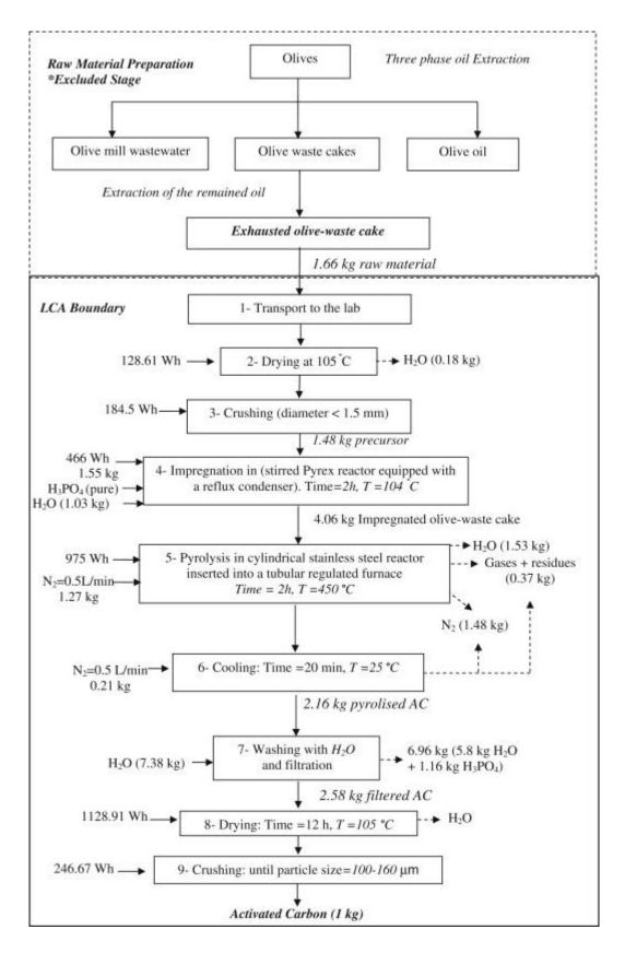
Figure 2.10 Production process flowchart to produce 1 kg of AC from olive-waste cakes [23]
